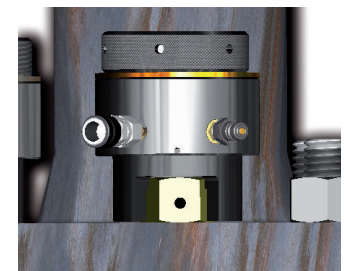
Once the target pressure is reached 'hold' the pressure and rotate the nut back down against the joint face. The bolt is loaded.
