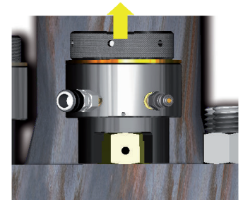
Assemble the bolt tensioning tool onto the bolt to be tensioned.
