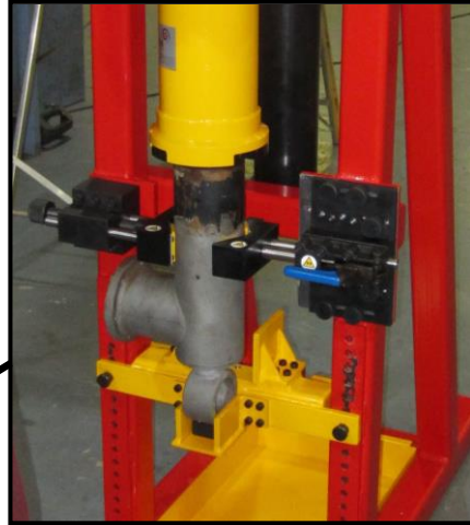
Drive socket fully engaged on drive adaptor and shock absorber
