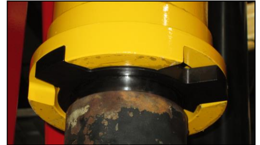
Drive socket fully engaged on drive adaptor and shock absorber
