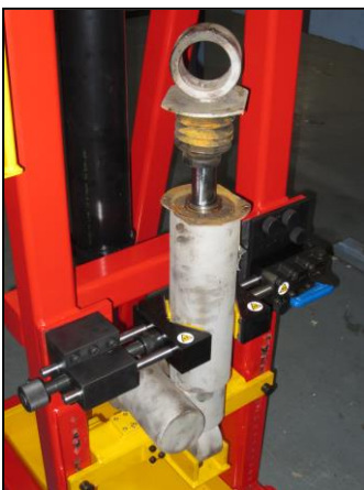
Shock absorber securely clamped in position
