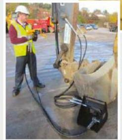
Hyspan PG powered from hydraulics of an excavator.
