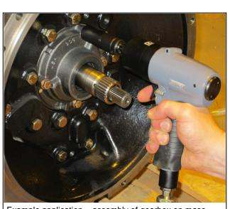
Example application – assembly of gearbox on mass production line
