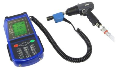
Optional Impulse Wrench Torque Checker Contact us for details
