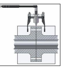
3) Engage the spreading bar through the leg of the tool and the flange stud hole.
