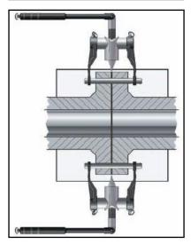
6) Turn each opposing tool a half turn at a time until the desired gap is achieved. Care must be taken to ensure the force is applied evenly. The maximum spreading distance for the WC7TM is 27mm.
