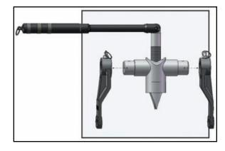
5) Drive the handle so that the splitter wedge moves down. Then remove the Splitter wedge and Thrust bearing from the tool.
