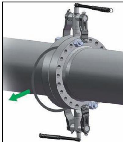
**Flange Spreading & Seal Removal**
