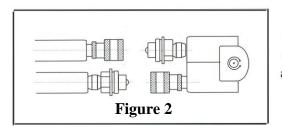
Ensure the connectors are fully engaged and screwed snugly and completely together.
