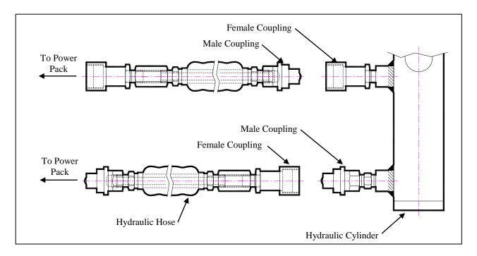
The LH tool and power pack are connected by a 10,000 psi (700 bar) operating pressure, twin-line hose assembly. Each end of the hose will have one male and one female connector to ensure proper interconnection between the pump and wrench.
