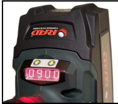
Figure 5.2-1: Torque Select Mode
